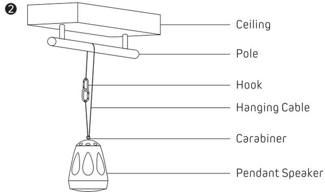
⚠ Make sure the speaker is properly secured to the ceiling / building's structure. please use the proper screws, bolts, or anchors (not included). Failure to do so may cause the speaker to become unsecured & cause potential damages/ injuries.
